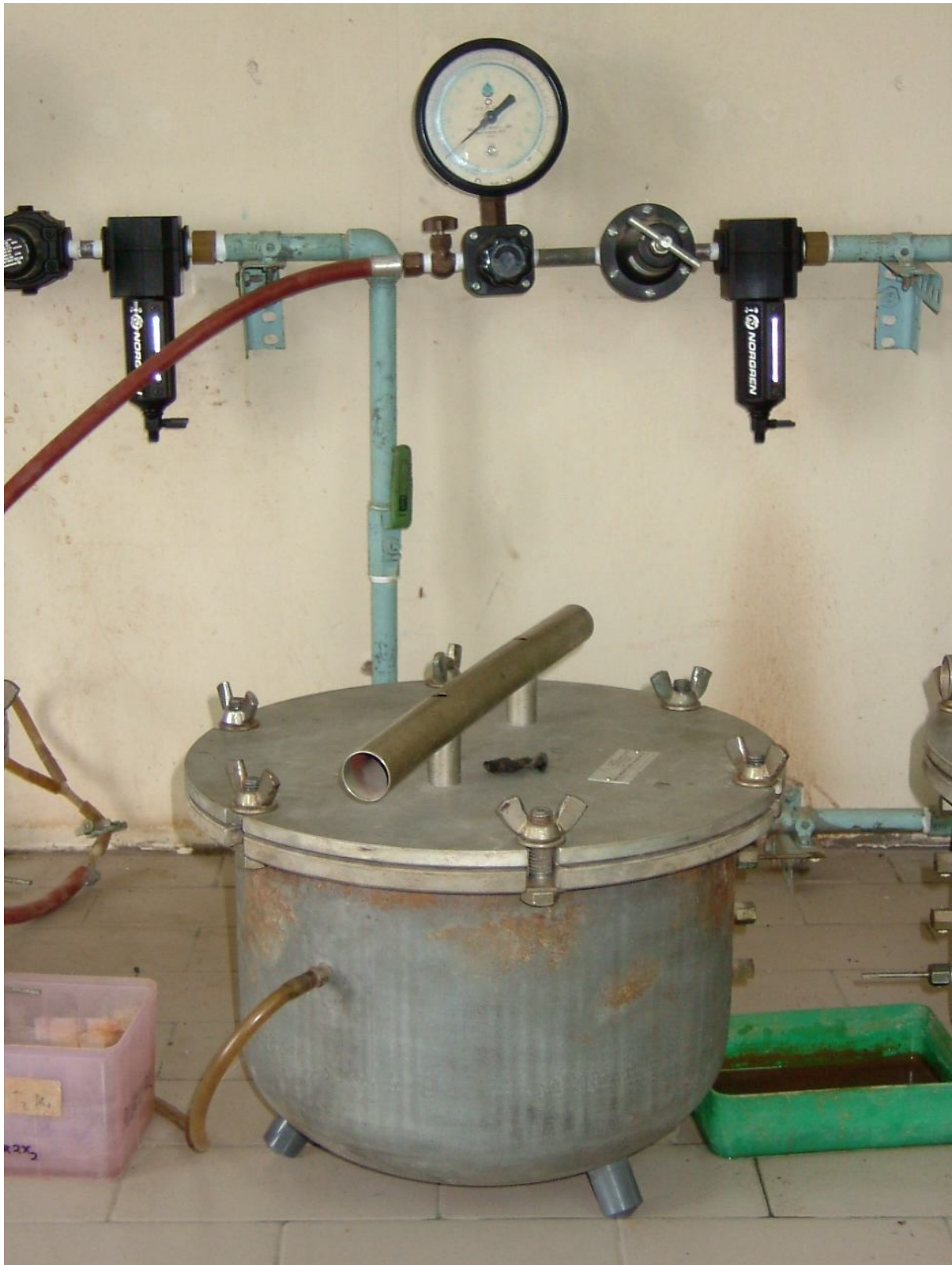
Figure 6. A pressure chamber to dry out a soil at a fixed constant suction
