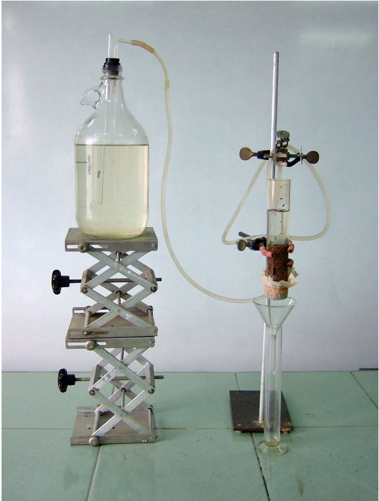
Figure 12. Measurement of saturated hydraulic conductivity
