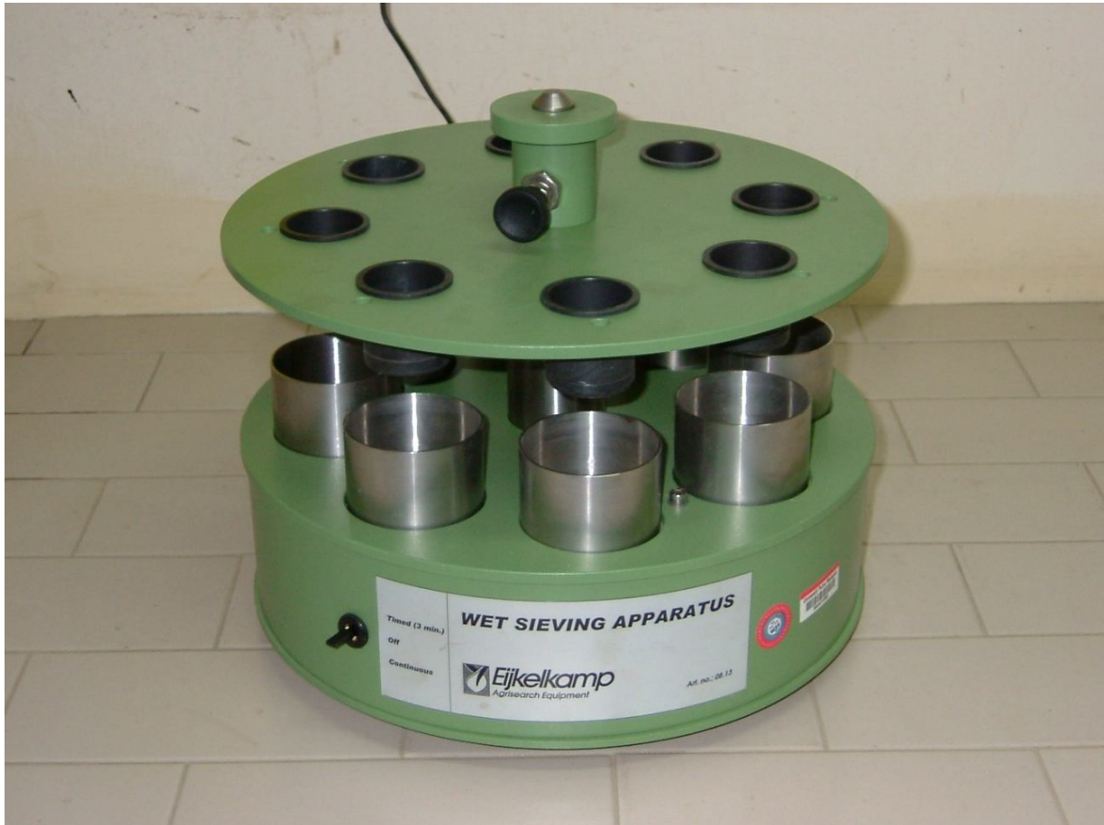
Figure 4. Wet sieving apparatus to determine aggregate stability
