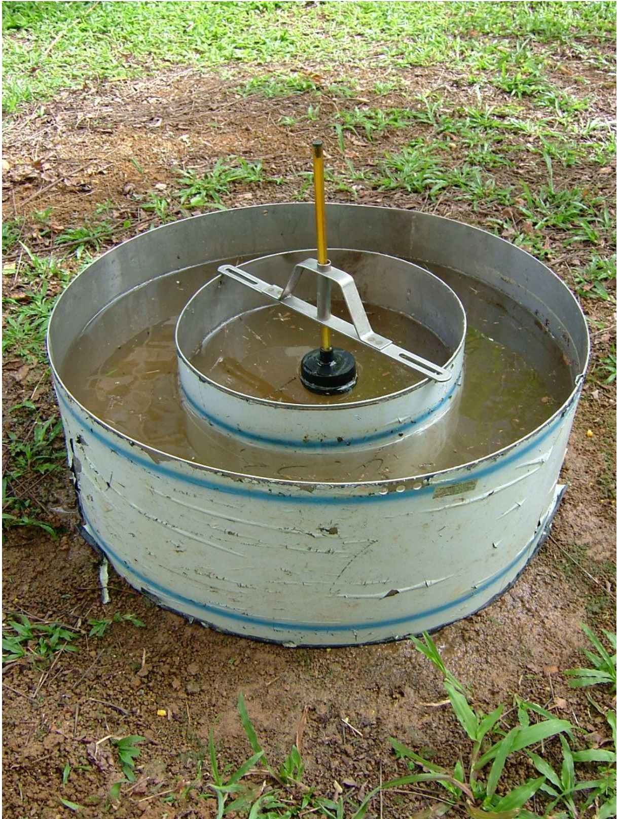
Figure 9. Double ring infiltrometer
