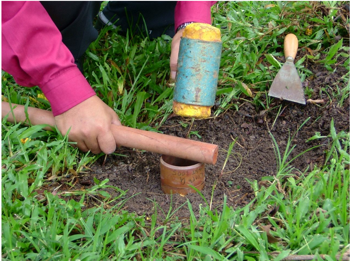
Figure 5. The core ring is hammered evenly into the soil
