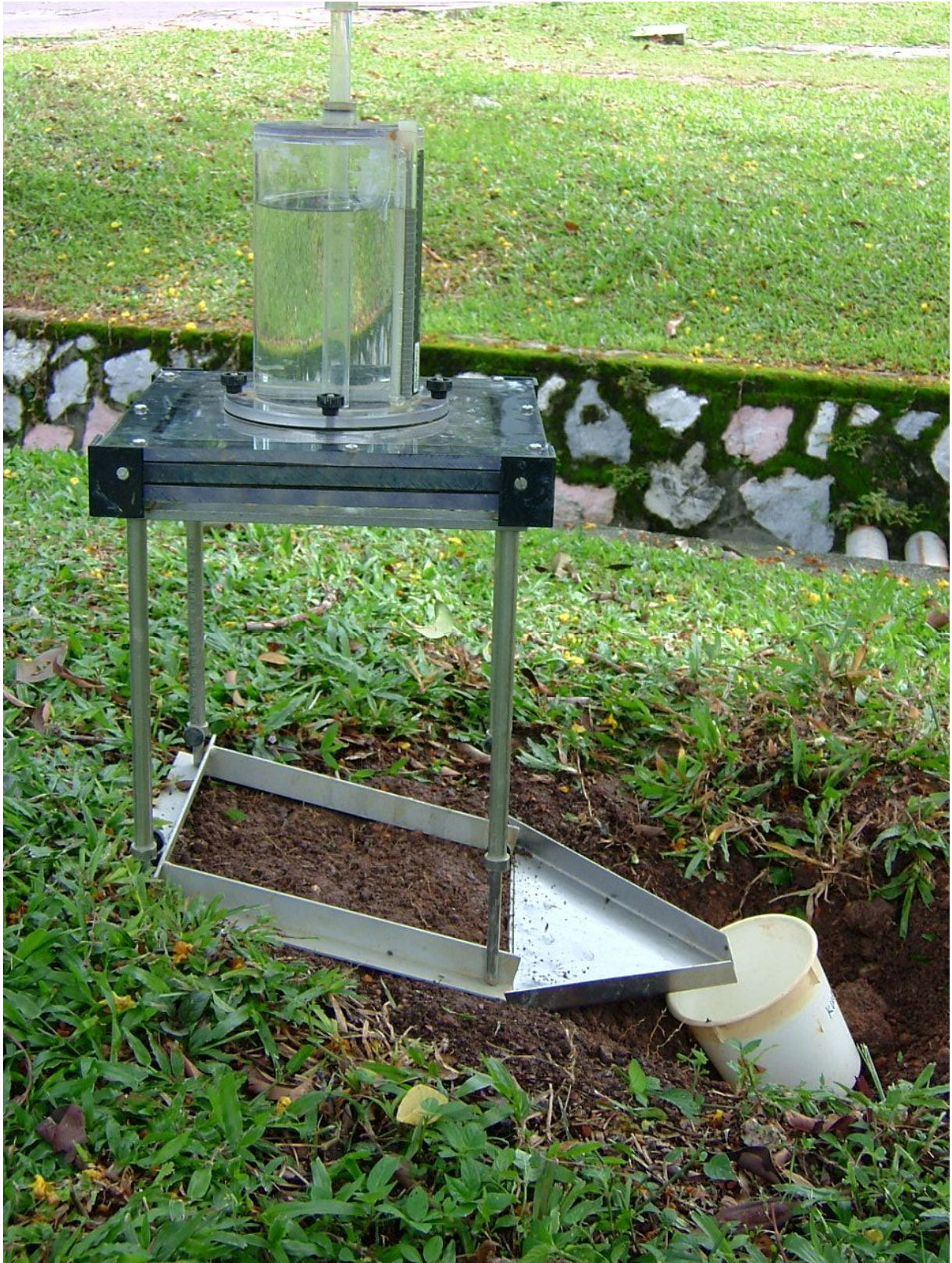
Figure 19. Rainfall simulator apparatus
