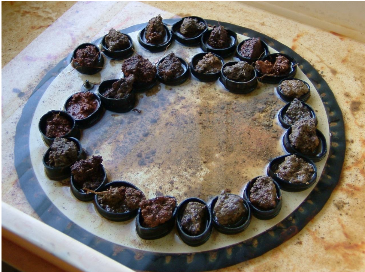
Figure 7. Soil samples and the ceramic plate are saturated
