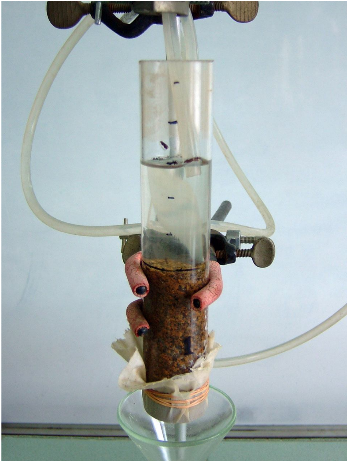
Figure 13. Close up of the soil column tube to measure saturated hydraulic conductivity
